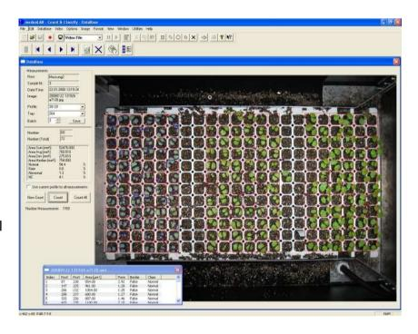
Automatic data import to lab PC via USB memory stick and analysis by medeaLAB Count & Classify software
