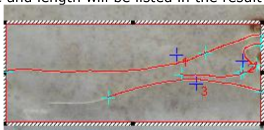
Root length measurement using the skeleton based method
